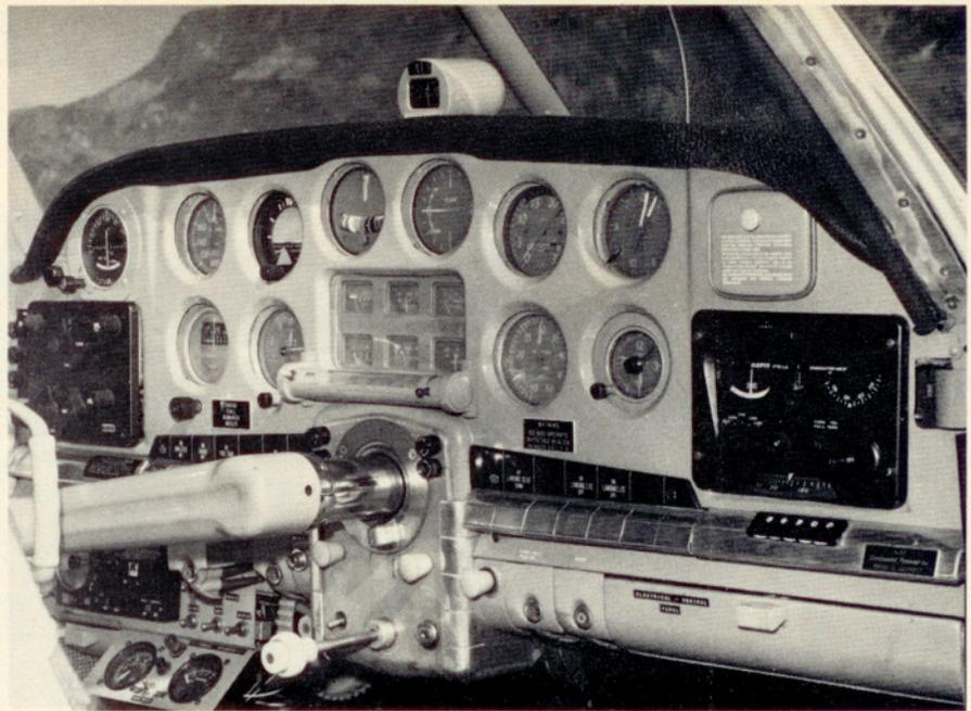
The panel of N202D belies the airplane's age, with older-style instruments spread about the panel and radios unfamiliar to many of today's pilots. That's a Narco Omnigator navcom on the right and a large King KX-100 navcom on the left with an also bulky King ADF just visible below it.
