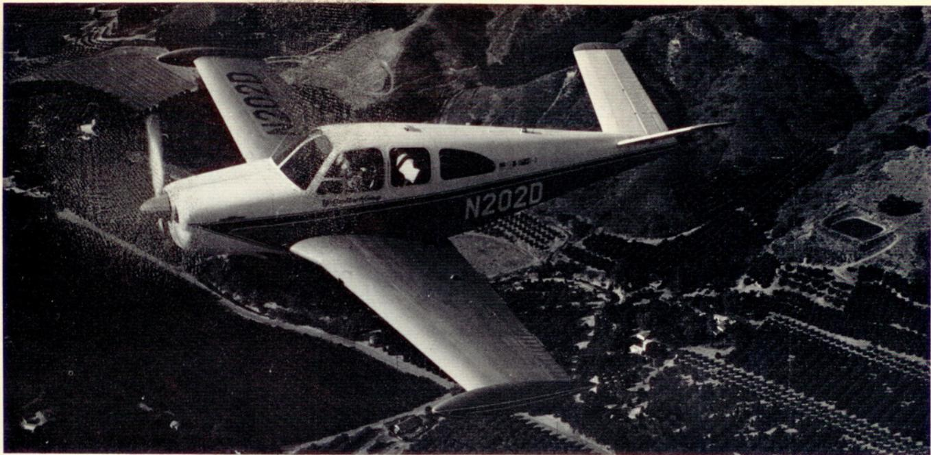
Many original Bonanzas have been modified and modernized by their owners. The one flown by the PILOT was no exception, with added third window, tip tanks—and a full paint job. Original stall warning vane remains on top of the left wing, just forward of the flap.
